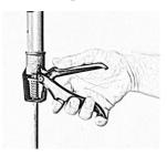
5.4 Check each actuator moves freely and free from interruption throughout its full operating range. An audible 'click' will transmit from the release catch when the system reaches its maximum permitted operating range. In this event cease operating the actuator immediately, press the release catch downwards and return the system to within its permitted operating range.
